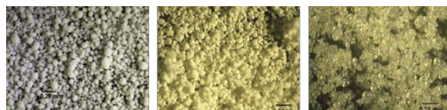
Figure 7: Image of Neusilin® US2 at various amount of cinnamon oil loading; left 0%, middle 62% & and right after 78% loading
